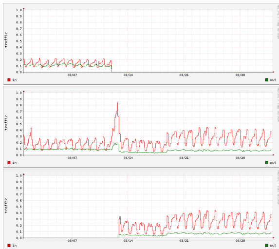
Traffic on 3 JP-US links for March 2011, damaged (top) not-damaged (middle) and rerouted (bottom)
