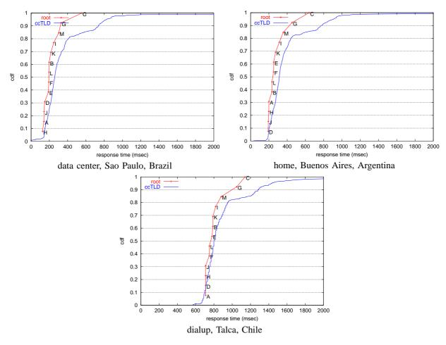
Fig. 19. median response time of root and ccTLD DNS servers (4/4)  $\,$
