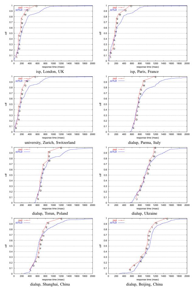
Fig. 17. median response time of root and ccTLD DNS servers (2/4)
