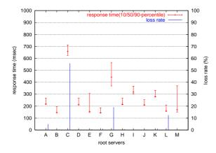
Fig. 3. measured response time and loss rate of the root servers
