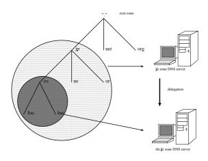
Fig. 1. The tree structure of Domain Name System
