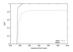
Fig. 7. comparison of the distribution of the response time by direct and dialup measurement of K-root
