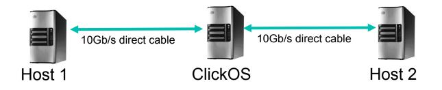
Intel Xeon E1220 4-core 3.2GHz (Sandy bridge) 16GB RAM, 2x Intel x520 10Gb/s NIC. One CPU core assigned to Vms, 3 CPU cores Domain-0 Linux 3.6.10
