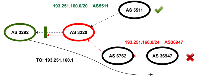
Figure 9: Collateral damage on AS 3292; ROV scores of AS 3292 and 3320 are 92.1% and 0% respectively.
